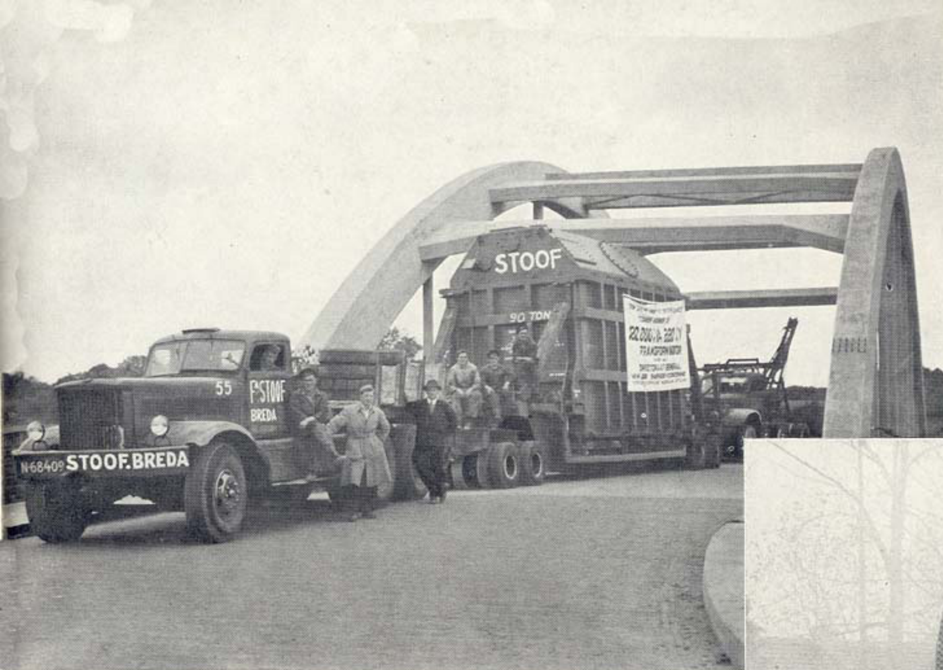
The transport of a boiler with a own weight of 45000 kg and 5 mtr high and a wide of 4 mtr.
