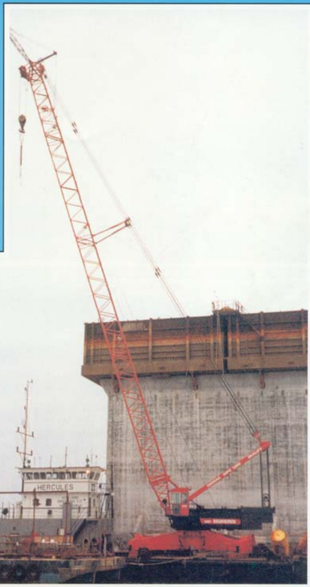
The crane is situated on the pontoon "Hercules" built up with a jib of 6 meter, maximum radius of 48 meter; 48 meter main boom and a counterweight of 50 tons.
