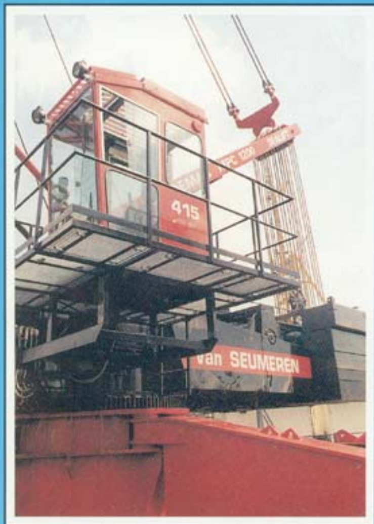
The crane is situated on the pontoon "Hercules" built up with a jib of 6 meter, maximum radius of 48 meter; 48 meter main boom and a counterweight of 50 tons.
